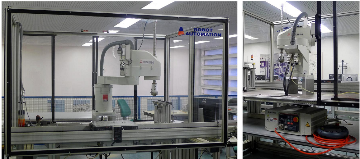
Fig. 4-29: SCARA robot cell under reconstruction with (front view and rear view)
