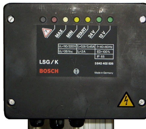
Fig. 4-25: Charging control unit
