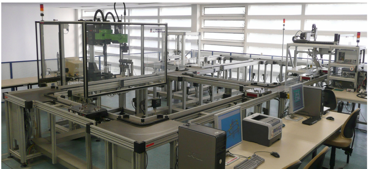
Fig. 4-1: Robot-based Flexible Assembly System (RFAS) at the UASA Hannover at project start
