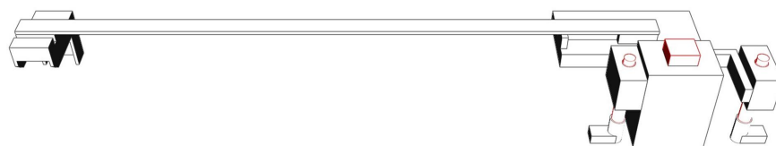
Fig. 6-9: CAD components – Stopper unit after simplification
